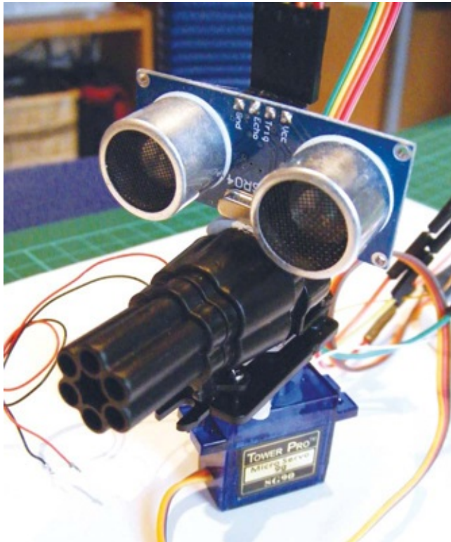
4. FIGURE 20-5: Attaching the ultrasonic sensor
